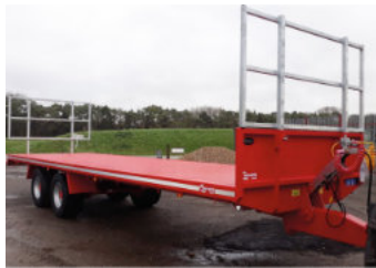
WARWICK BALE TRAILER AIR/HYD BRAKES, LOAD SENSING - £12,250
