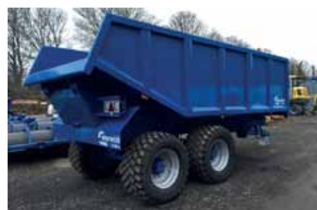
Warwick 14 Tonne High Dump Trailer NEW STOCK Parking Brake, 550 x 45R, x 22.5 Floatation tyres, LED Lights, Two Year Warranty £13,950
