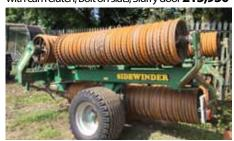
**Cousins Sidewinder** Horizontal Folding 5 gang 12m Hydraulic Folding Rollers, 22 inch Cambridge breaker rings, in good order **POA**
